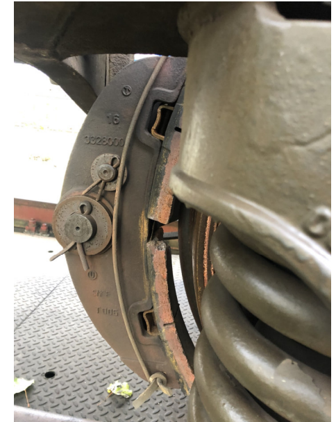
Change of color of the brake block
