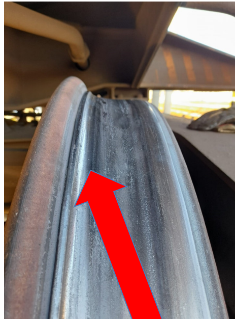
Extraordinary wheel tread deformation near the flange
