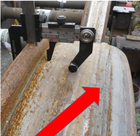
Extraordinary wheel tread deformation on the outer side of the tread
