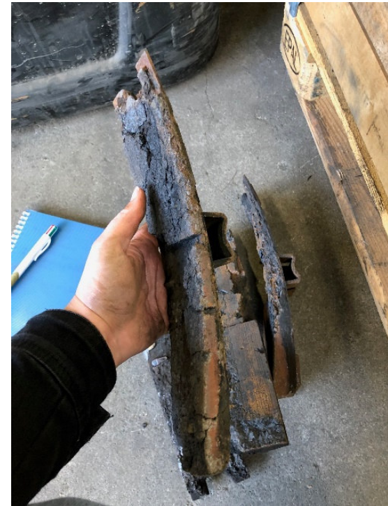
Carbonized brake block
