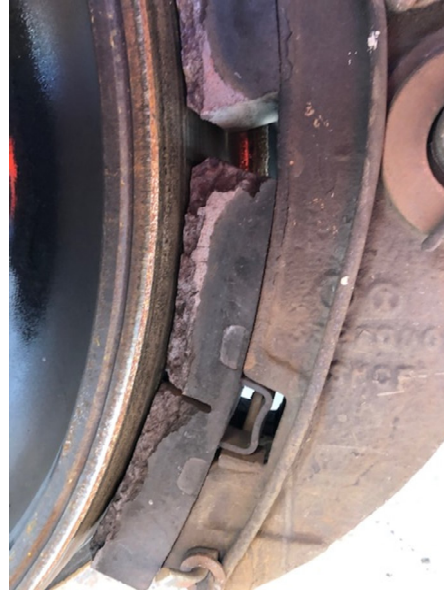
Change of color and broken out brake block material
