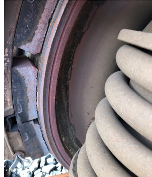
Change of color on the brake block and burned paint on the rim web transition of the wheel
