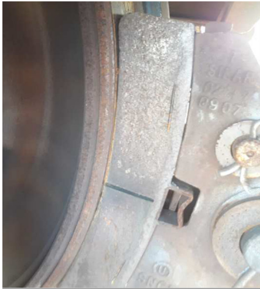
Brake block in normal conditions
