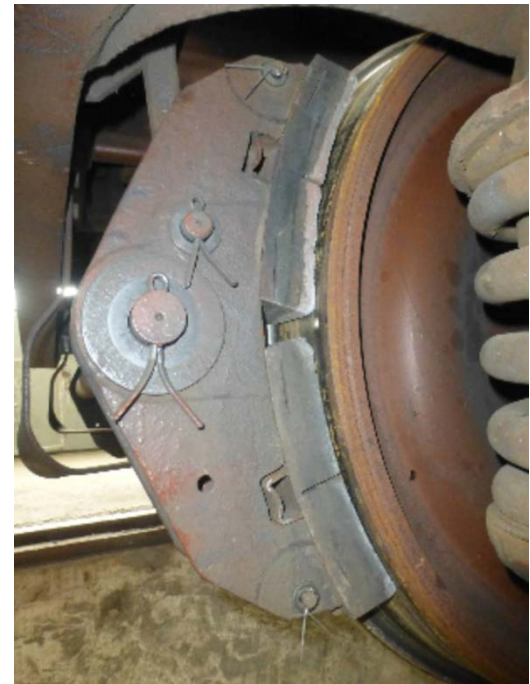
Melted brake block
