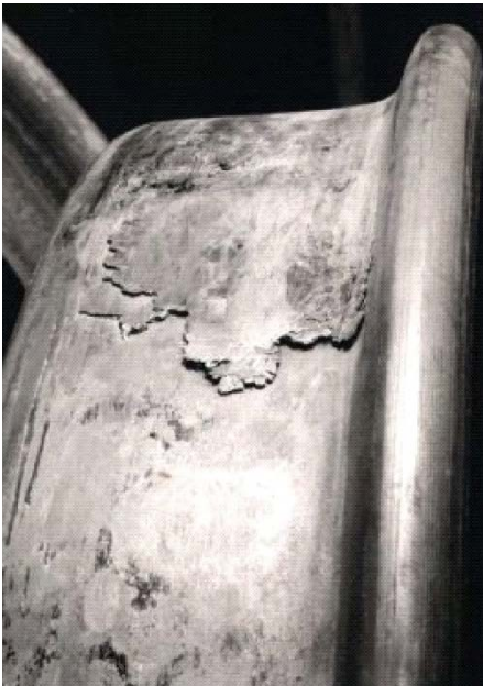
Metal build up on the tread
